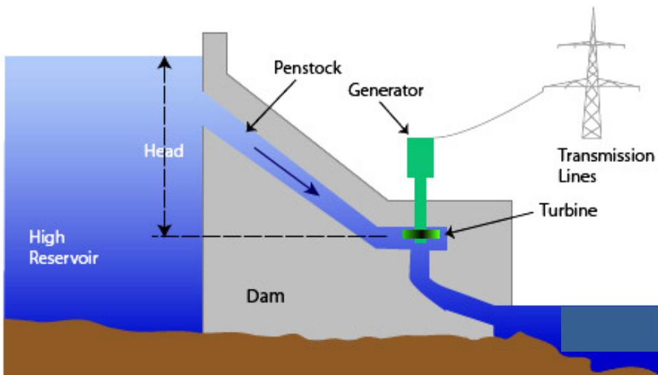
Potential energy of water in reservoir is passed through Penstock to a water turbine. Potential Energy of water is transferred to mechanical rotation by means of water turbine. A shaft coupled with turbine rotates the Generator and electricity is produced.
