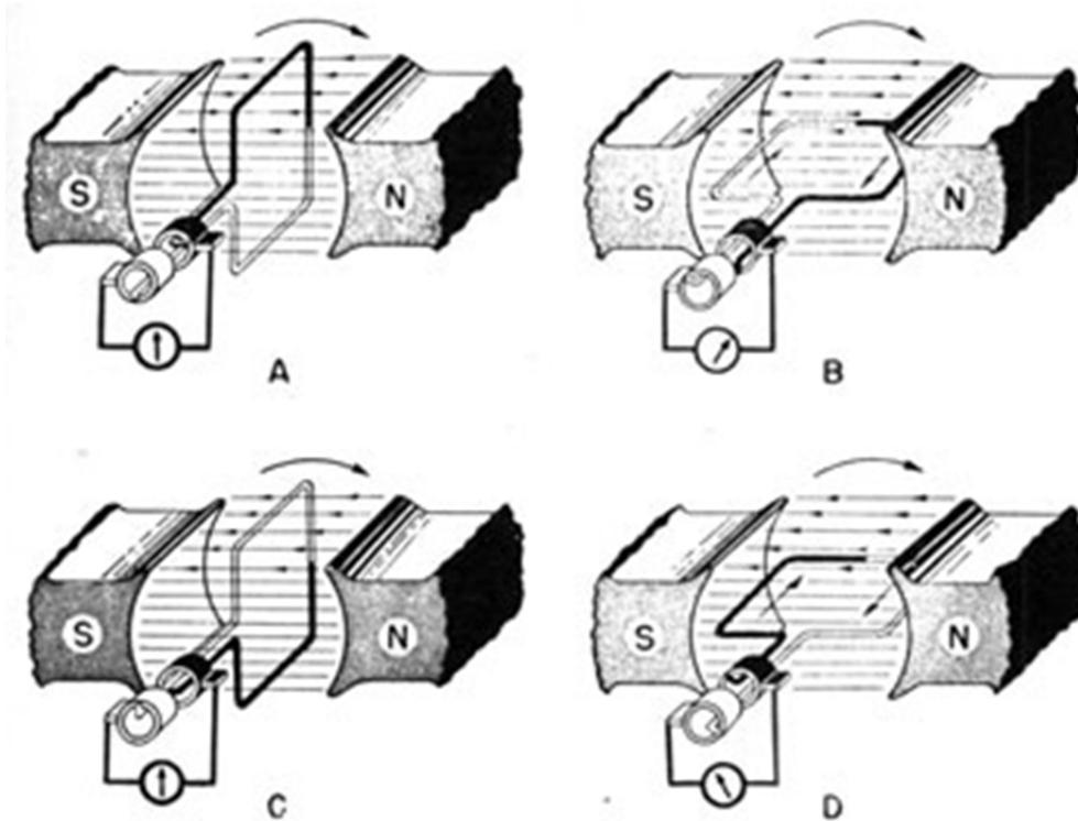
When coil is at vertical position (A) i.e. motion of the coil is making an angle  $\theta = 0^\circ$  to the direction of magnetic field, the change of flux linkage is zero and hence the induced emf is also zero. As the coil rotates flux linkage increase till the angle becomes  $\theta = 90^\circ$ . In this position the rate of change of flux linkage is maximum. The direction of induced emf is given by Fleming's Right hand Rule.
