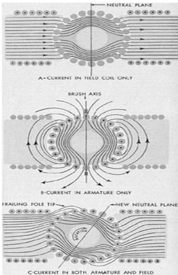
There are two kinds of magnetic fluxes acting in DC Generator; the first one is because of the stator poles called main flux, while the second one is because of the current flowing in the armature called armature flux. The effect of armature magnetic field setup by armature current on main magnetic field is called armature reaction. Armature reaction weakens as well as distorts the main flux, thus the overall effective flux in DC Generator decreases.
