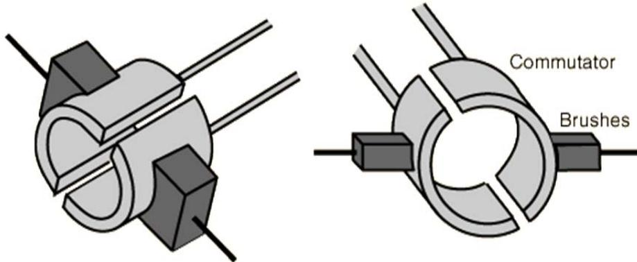
Brushes ride on the commutators and collect(or supply) current from (or to) Armature conductors. They are made of carbon and held in contact with the commutator by using spring.
